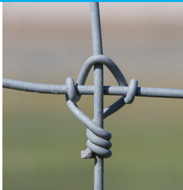
Fixed Knot: A locking fixed knot ties the vertical stay wires and the horizontal line wire together, providing maximum strength up to 1,385 pounds of pressure.
